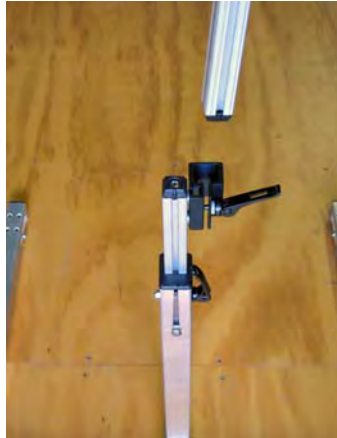
Line up the post slot with the clamp slot, and insert the Post
