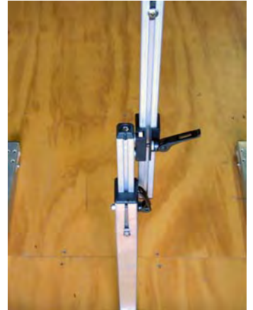
Drop it down to the height set screw Adjust the Floor Stand height if needed
