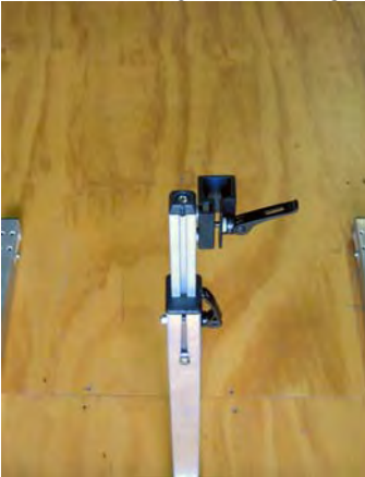
Make sure the Floor Stand clamp is unlocked
