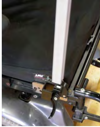
Unlock the wheelchair bracket clamp
