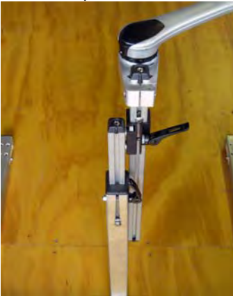
Make sure the Floor Stand clamp is unlocked
