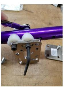
Once you have an Adapter Plate and the Coved Spacers secured, you can attach the Wheelchair Bracket directly to the plate or use additional Adapter Plates or an L-Angle extension plate to offset the placement of the Wheelchair Bracket and post. This can help avoid brake levers, footrest levers or armrests.
