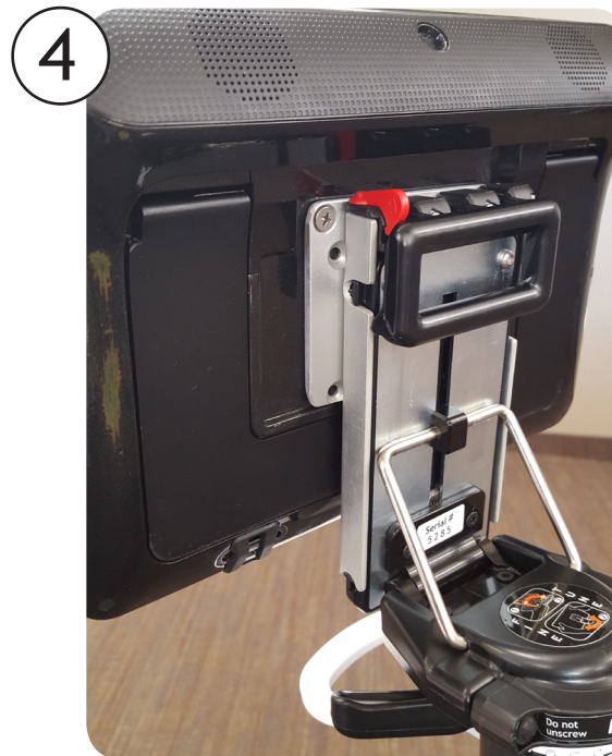
You can locate the Tobii device higher or lower on the Quick Release Plate depending on your preference
