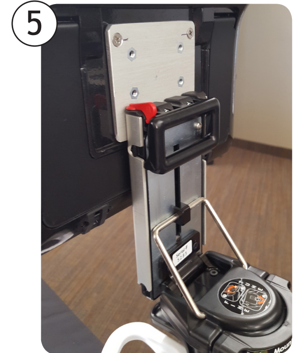
You can locate the Tobii device higher or lower on the Quick Release Plate depending on your preference
