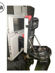
Attach the QRP to the Tilt Plate on the Mount'n Mover arm.
