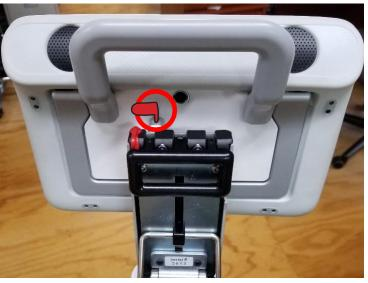
Locate the release lever (circled in red)
