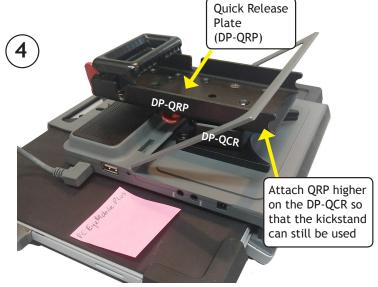
Attach the Quick Release Plate (QRP) to the DP-QCR. Use 4 screws provided with the QRP (8-32-1/4") "QRP to Device Plate"
