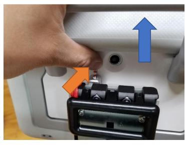
While depressing the lever, pull up on the device for removal.
