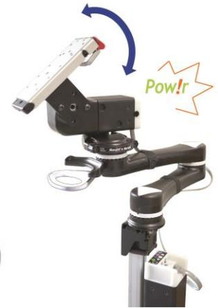
Unique mechanisms allow users to independently manipulate the attached device with great ease and flexibility.
