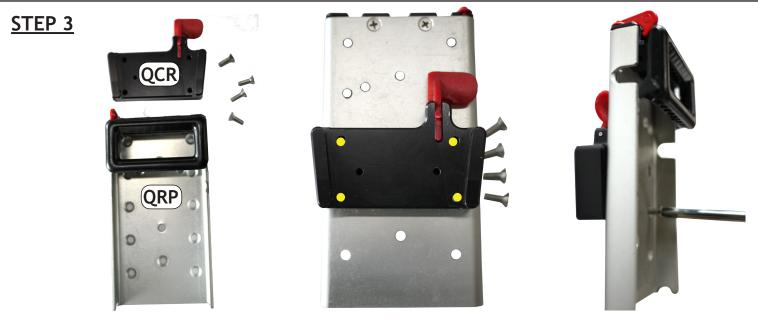
Quick Connect Receiver (QCR) and the Quick Release Plate (QRP). Attach the QCR to the QRP with four screws (8-32 x 1/2 inch) included with the Quick Connect Receiver.
