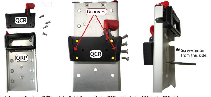
Quick Connect Receiver (QCR) and the Quick Release Plate (QRP). Attach the QCR to the QRP with four screws (8-32 x 1/2 inch) included with the Quick Connect Receiver.  $\bigstar$  Note the grooves on the QCR
