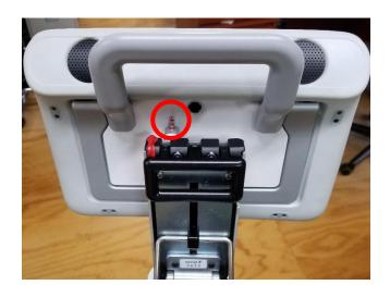
While depressing the lever, pull up on the device for removal.
