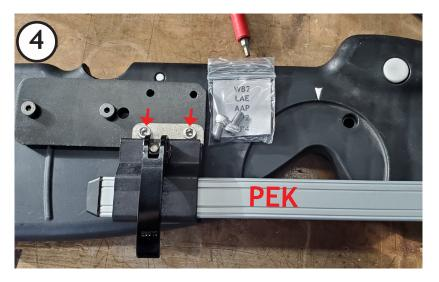
Attach the PEK (post extension kit) to the threaded holes on the WC-AP8X using two socket head 1/2 inch bolts (included).
