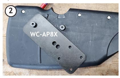
Attach WC-AP8X adapter plate using longer shoulder bolts (included). Once one longer bolt is in, then remove the other Rifton bolt and attach the WC-AP8X with two longer shoulder bolts. Use a *4mm allen wrench* to tighten.
