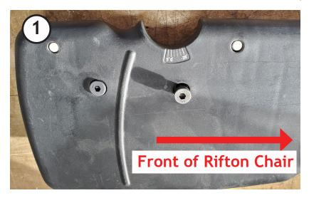
Remove one shoulder bolt from Rifton side panel. Use a *Torx 25 wrench* to do this. Do not remove both at once or the side panel may fall off.
