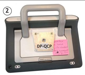
Place the DP-QCP plate over the spacers and use the two M4-16 screws to attach it to the back of the device.
