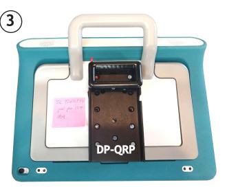
Attach the Quick Release Plate (QRP) to the DP-QCR using the four screws included with the DP-QCR labeled HS-Screw-X (8-32 x 1/2")
