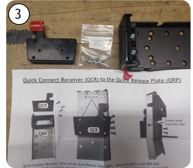
Attach Quick Connect Receiver to Quick Release Plate. See step #4 for holes to use on QRP
