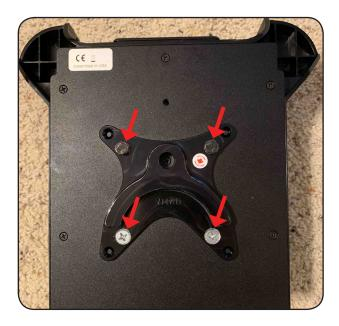
Remove four screws holding on the Daessy Bracket. Remove the Daessy Bracket.
