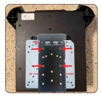
Attach the Quick Release Plate (QRP) to the Multi Plate using four 8-32 x 1/4" screws labeled "QRP to Device Plate"
