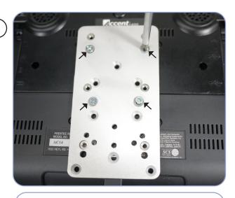
Place DP-PRC1 over the Accent 1400 mounting bracket. Line up the four holes between the two plates and the Accent 1400. Attach using the four screws provided (6/32 x 1/2").
