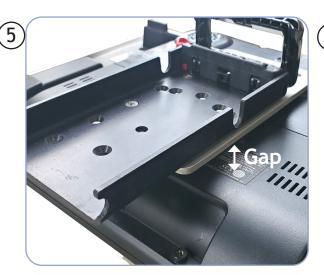
There should be a gap between the DP-PRC1 plate and the Accent 1400 to allow for ventilation.
