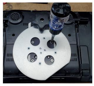
Spin the rotator to locate the holes in the attached (black plate). Use the screws "Rotator to PRC1 plate" to attach rotator.
