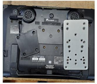
Remove PRC mounting bracket. Use same screws to attach PRC1 plate (silver plate).
