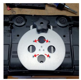
Straighten out the rotator and attach the QRP (quick release plate) to the threaded holes on the rotator.
