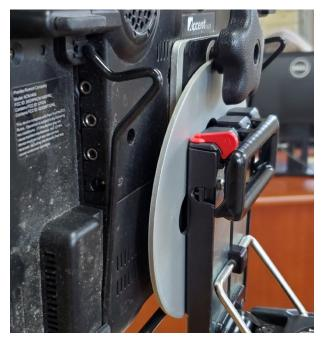
All attached and mounted. Loosen the knob on the rotator and spin to adjust the angle. Tighten when angle is correct! pg 2 of 3
