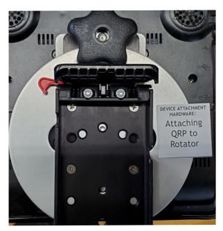
Be sure to use the screws "attaching QRP to Rotator". If you use too long of screws the rotator will not spin. (8-32 x 3/16)
