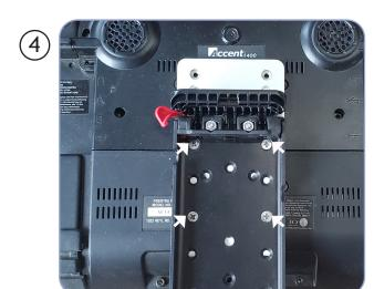
Attach the Quick Release Plate to the DP-PRC1 using the four screws provided (8/32 x 1/4")
