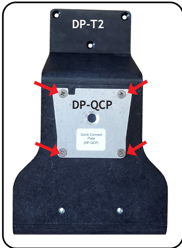
Attach the DP-QCR to the DP-T2 with four screws (8-32 x 3/8th inch)
