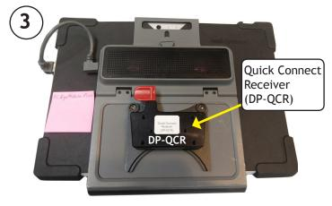
Slide the DP-QCR onto the Quick Release Adapter Plate until it "clicks" and locks in place.
