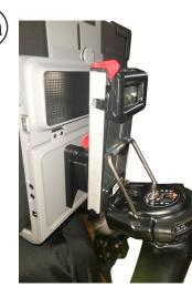
Attach the QRP to the Tilt Plate on the Mount'n Mover arm.
