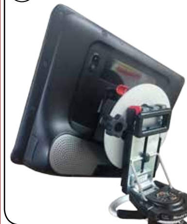
Attach the QRP to the threaded inserts on the DP-UR with four screws (8-32 x 3/16") labeled "QRP to Rotator".
