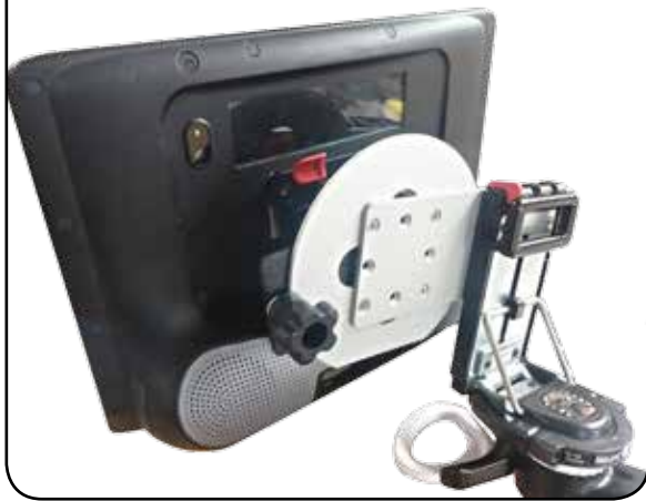
Rotator used with Extension plate for access to Infrared window.
