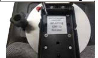
Attach the QRP to the threaded inserts on the DP-UR with four screws (8-32 x 3/16") labeled "QRP to Rotator".
