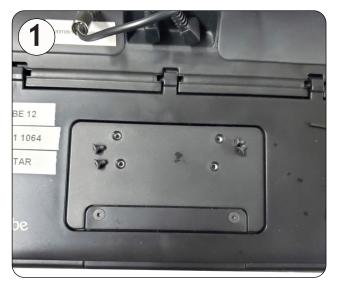
Back of Vibe 12. Remove small screws from plate. Leave plate in place.
