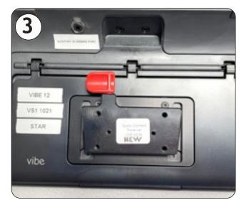
Attach the DP-QCR (Quick Connect Receiver) to the Tobii mounting bracket. Red pin should "click" into the bracket
