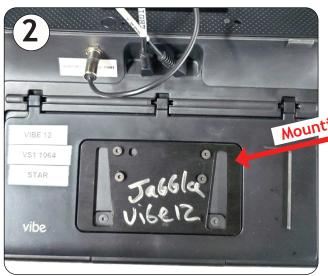
Attach the mounting bracket provide by Jabbla. Use the longer screws that come with the bracket.
