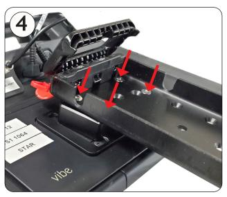
Attach the Quick Release Plate to the DP-QCR using four screws 8-32 x 1/2" included with the DP-QCR
