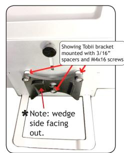
Attach the Tobii quick release adapter plate using the hardware labeled "Tobii Eyemobile Mini Offset Hardware". Place the nylon spacers over the threaded holes on the back of the Tobii bracket. Use the M4x16 screws to attach the quick release bracket.
