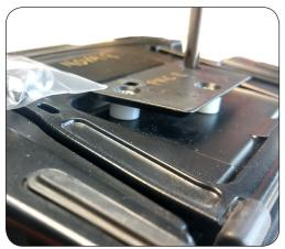
Close up view of the spacers underneath the attachment plate.
