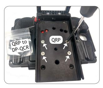
Place the QRP over the QCR and attach with the four screws labeled "QRP to DP-QCR"
