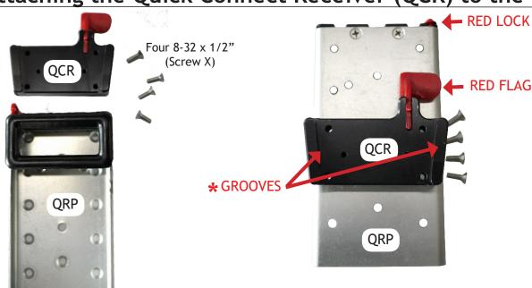
Quick Connect Receiver (QCR) and the Quick Release Plate (QRP) and hardware four screw X. Line up four holes in the QCR with corresponding holes in the QRP. ★ Note the grooves in the QCR are facing out. The red lock on the QRP and the red flag on the QCR are facing up.
