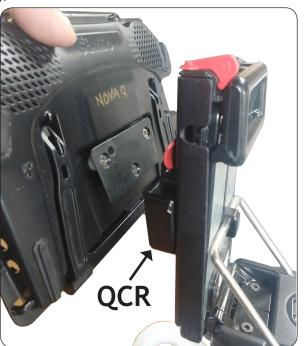
Remove the Nova Chat 8 from the Mount'n Mover at either the QCR (Quick Connect Receiver) or the QRP (Quick Release Plate).
