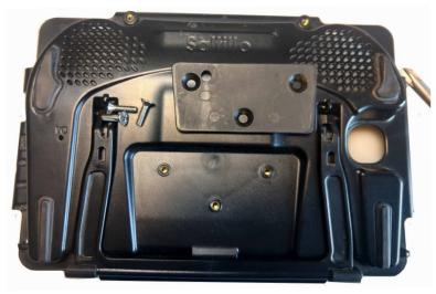
Remove the screws and plate from the back of the Nova Chat 8
