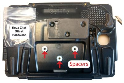
Use spacers and screws from hardware bag labeled "Nova Chat Offset Hardware". Place spacers over threaded holes.
