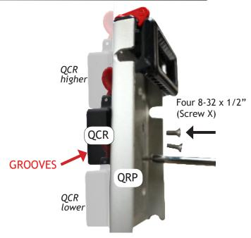
Feed the four 8-32 x 1/2" screws through the inside of the QRP and into the back of the QCR. The hole spacing in the QRP allows adjustment higher or lower depending on preference
