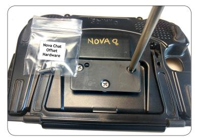
Place plate over the spacers and reattach to the back of the Nova Chat 8 with the longer screws included in the hardware bag.
