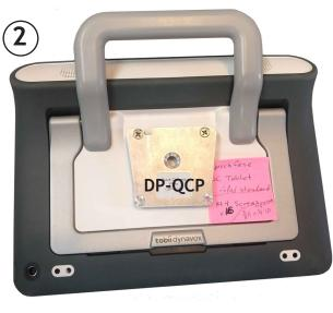
Place the DP-QCP plate over the spacers and use the two M4-16 screws to attach it to the back of the device.
