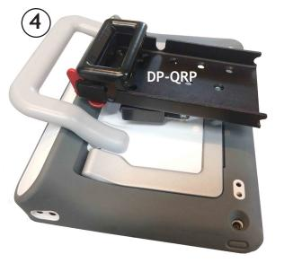
Attach the QRP onto the DP-QCR with the four screws included with the DP-QCR (HS-Screw-X {QRP to DP-QCR})
