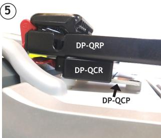
Close up of QRP attached the the DP-QCR attached to the DP-QCP.
