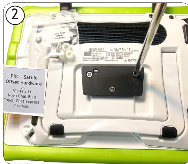
Re-attach the PRC plate over the spacers using the three screws provided "PRC-Salttillo offset hardware" (6-32 x 1/2")
