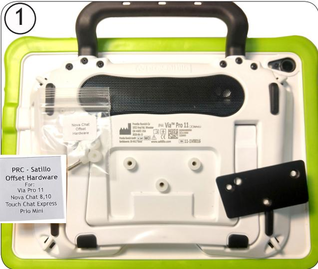
Remove black PRC attachment plate. Place three 3/16" spacers over the holes.
