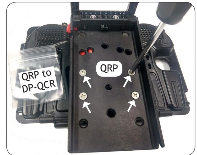
3 Place the QRP over the QCR and attach with the four screws labeled "QRP to DP-QCR"
