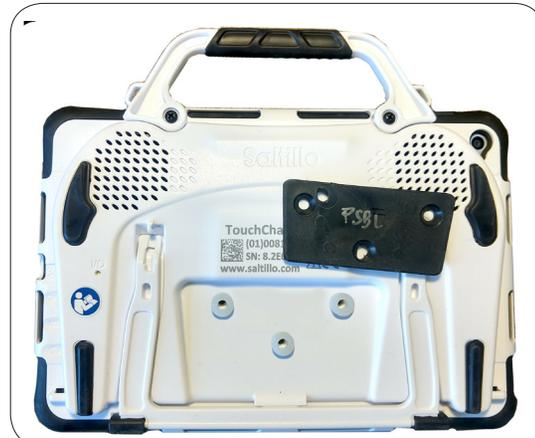
Remove black plate, place spacers, reattach with longer screws (6-32x1/2")
