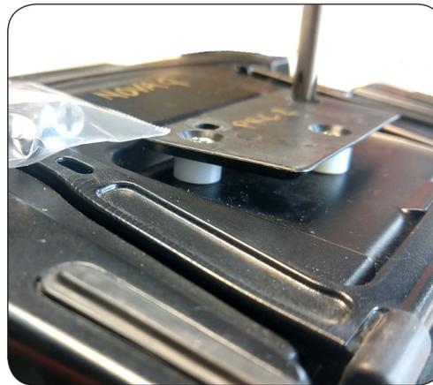
Close up view of the spacers underneath the attachment plate.
