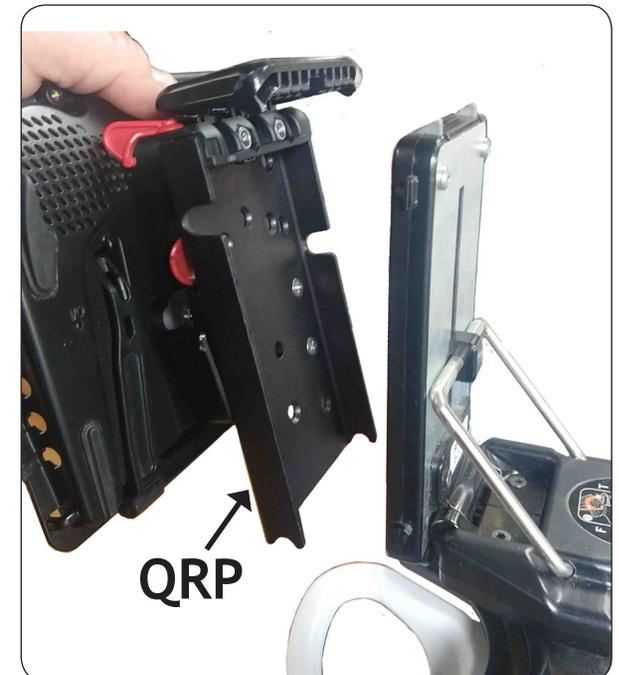
\* Remove the Nova Chat 8 from the Mount'n Mover at either the QCR (Quick Conect Receiver) or the QRP (Quick Release Plate).
