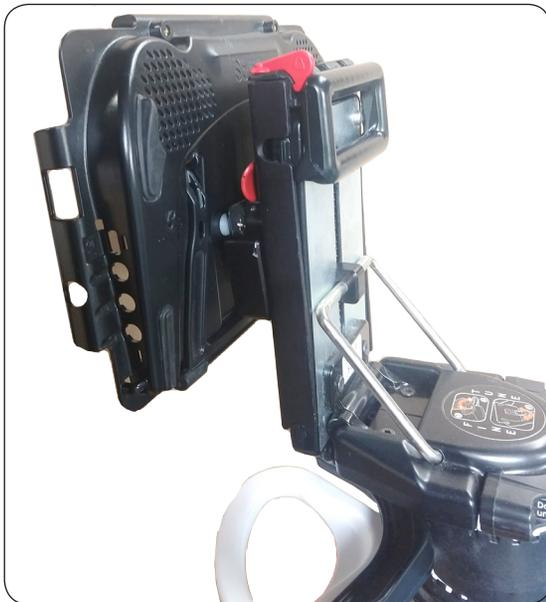
4 Nova Chat 8 attached to the Dual Arm Mount'n Mover with Tilt Plate
