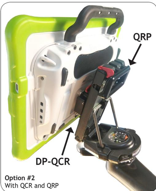
Showing the QRP (Quick Release Plate) attached to the QCR (Quick Connect Receiver) and then to the Via Pro 11
