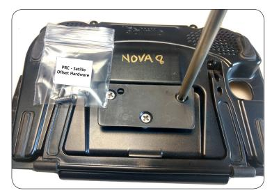
Place plate over the spacers and reattach to the back of the Nova Chat 8 with the longer screws included in the hardware bag. (6-32 x 1/2")
