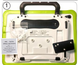
Remove black PRC attachment plate. Place three 3/16" spacers over the holes.
