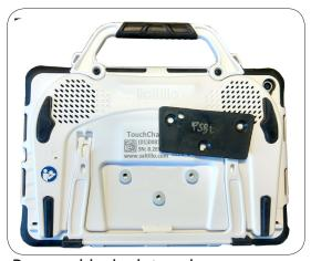
Remove black plate, place spacers, reattach with longer screws (6-32x1/2")
