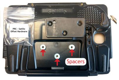
Use spacers and screws from hardware bag labeled "PRC-Saltillo Offset Hardware". Place spacers over threaded holes.
