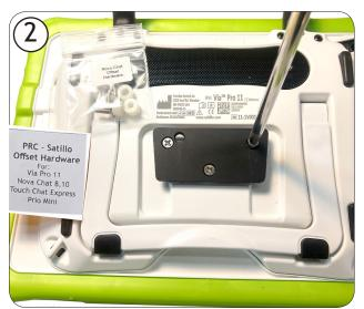
Re-attach the PRC plate over the spacers using the three screws provided "PRC-Saltillo offset hardware" (6-32 x 1/2")
