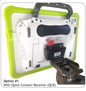
Showing the DP-QCR (Quick Connect Receiver) attached to the Via Pro 11
