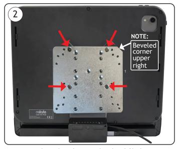
Attach Multi Plate to back of Skyle device using four m4 x 10mm screws (included).
