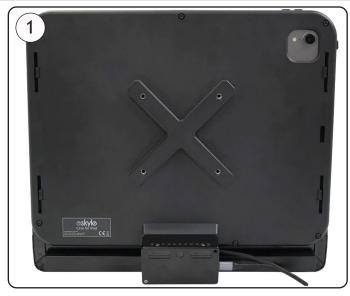
Back of Skyle has 75 VESA hole spacing. The thread size is m4 x 10mm (x4).
