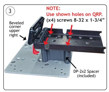
Use four 8-32 x 1- 3/4 inch screws (included) to attach the Quick Release Plate, through the DP-2x2 Spacer and into the threaded holes in the Multi Plate.
