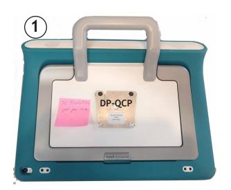
Place the DP-QCP plate over the two threaded holes on back of device. Use the two M4-10 screws included with the DP-QCP to attach it to the back of the device.
