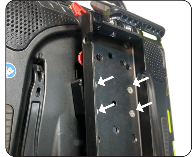
Attach Quick Release Plate (DP-QRP) to Quick Connect Receiver (DP-QCR) using four 8-32 x 1/2 inch screws (included with DP-QCR).
