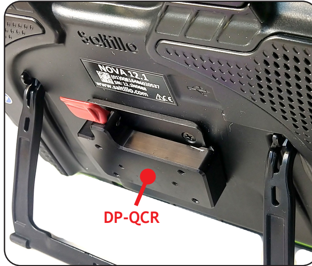
DP-QCR (Quick Connect Receiver) attached to the mounting bracket
