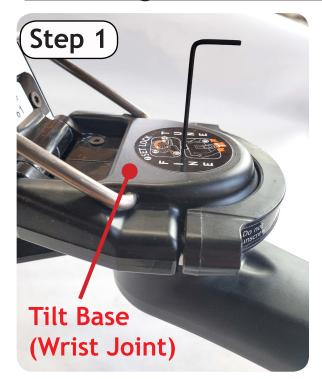
Poke a hole through center of sticker with 1/16" hex wrench. Locate fine tuner screw with the wrench end.
