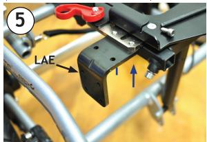
Attach LAE plate to the AP4 plate using provided screws
