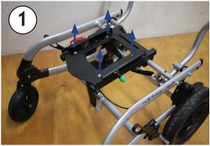
Remove four flat head screws and nuts securing the seat bracket to the base.
