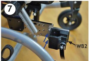
Attach WB2 to the AP2 plate using the provided screws
