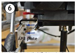
Attach AP2 plate to the LAE plate using the provided screws
