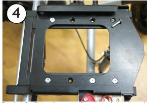
Sandwich AP4 and spacers between the seat and base. Fasten together using five M6 x 25mm flat head screws into M6 lock nuts (provided)
